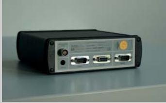
Back side of v10dsp with CAN-Bus and RS232 interfaces
