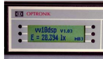
LCD integrated in preamplifier vv10dsp
