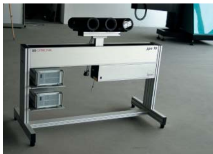
LMS20 in automated application with PPE10 automatic photometer positioning unit
