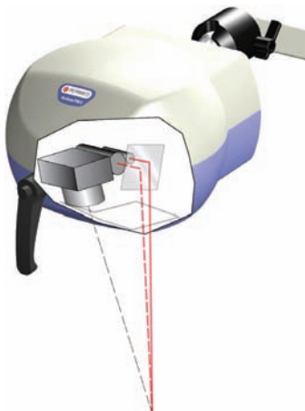
Principle of PeriScan PIM 3 System.
