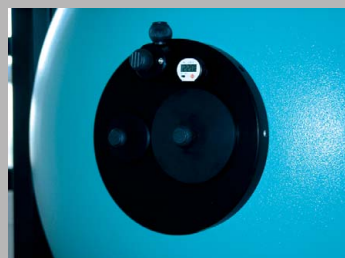
Detector ports for flux and luminous color measurement, thermometer
