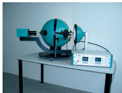
KMS10—transmittance and reflectance measurement instrument
