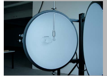
Internal view: three burning positions, up-side, down-side (vertical), front-side (horizontal)
