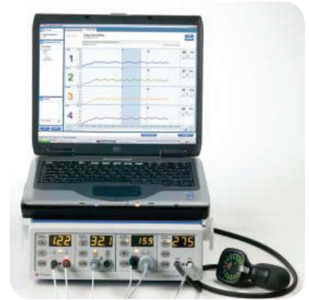
PeriFlux System 5000 equipped with PF 5010 Laser Doppler Unit, PF 5020 Temp Unit, PF 5040 tcpO 2 and PF 5050 Pressure Unit.
