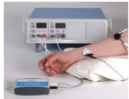
Iontophoresis in combination with blood perfusion monitor PeriFlux System 5000.
